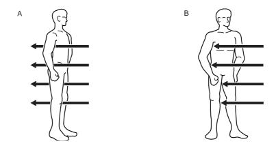
The laser light is emitted from the right side. This means that if your aim is to capture the void between the legs, for example, it is best to mount the doll so that it faces right. The direction in which the laser light is incident is decided by the orientation of the scan object mounted on the table. With multi-plane composition, this orientation is the first surface for scanning.
